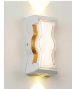
Item No.:MGW19339-2A Material:Aluminum+Acrylic Size:160*102*55mm Power:3W*2+5W single color
