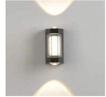
Item No.:MGW19335-2B Material:Aluminum+Acrylic Size:95*45*58mm Power:1W*2+2W single color
