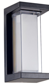
Item No.:MGW4964-1 double PC shade Material:Aluminum+PC Size:260*125*125mm Power:18W single color
